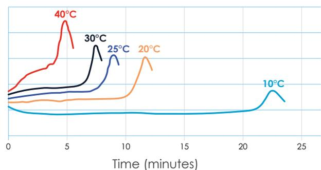
Figure 4: At higher ambient temperatures the working time for MMA adhesives is reduced.
