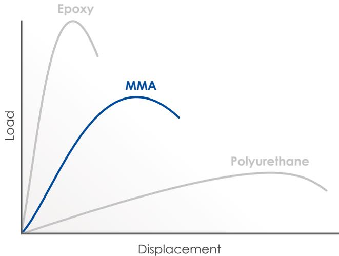
Figure 2: As this chart of load (strength) against displacement (elongation) illustrates, MMA technology bridges the gap between the tensile strength of epoxies and the flexibility of polyurethanes.
