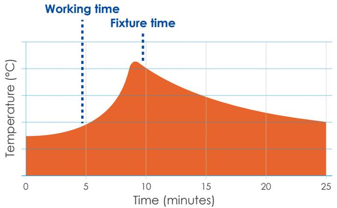
Figure 3: This graph of exotherm temperature vs time at room temperature shows the fast cure of an MMA adhesive.
